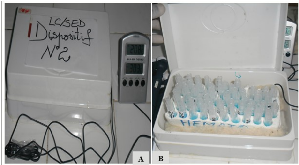
Figure 2. Experimental device 2 designed to substitute the room temperature provider. Device 2 seen from the outside (A) and from inside (B), composed of a plastic, hermetic and opaque box of size 22cm x 14cm x 8cm containing an ice pack.
