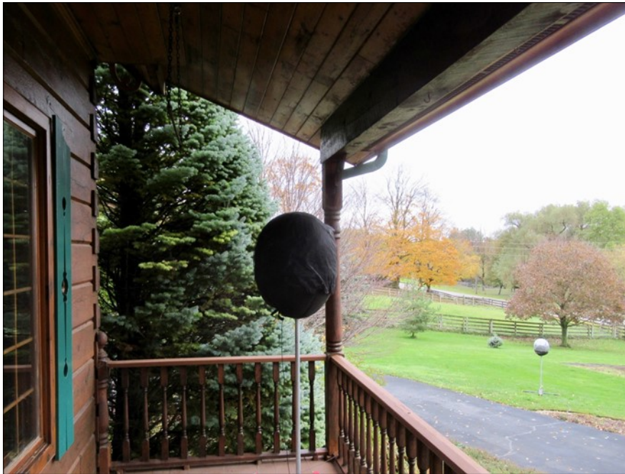
Figure 6. Microphone Test Locations for Free-Field and Covered Porch
