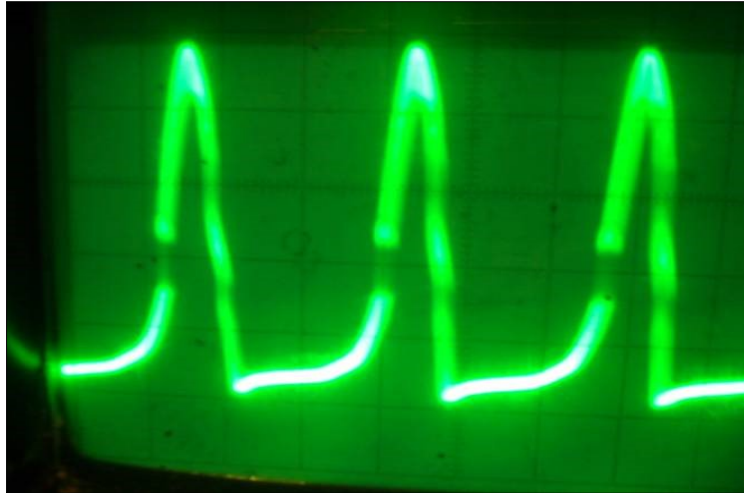
Figure 18. Oscillograph of the collector voltage in the physical model of the system (7) corresponding to the solution of the KdV equation. Vert axis milli sec/cm , Horiz axis-3volts per cm.
